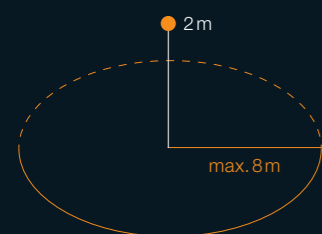
Mounting height 2 m Detection zone Ø max. 16 m
