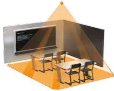
Classroom situation, detection by the Presence Control Pro IR Quattro with square detection characteristic
